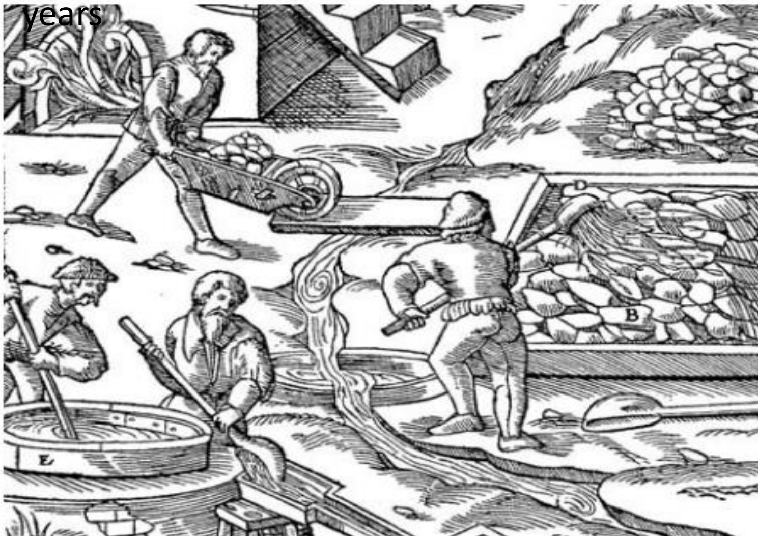
Figure 1. "The rocks are . . piled in . . heaps fifty feet long, eight feet wide and four feet high, which are sprinkled for forty days with water. The rocks begin to fall to pieces like slaked lime, and there originates a . . new material". Drawing and text from De Re Metallica , Herbert Hoover translation, published by Dover Publications, Inc.
