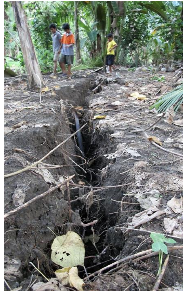
Lateral spread that appeared in Brgy. Tamlangon after the M6.6 earthquake that has worsened after the M6.5 earthquake
