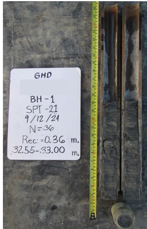
SPT sample showing dense material at 32 m
